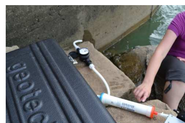
CDC laboratorian uses dead-end ultrafiltration to obtain a high-volume water sample
